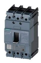
circuit breaker 3VA5 UL frame 125 3-pole, starter protection TM120M, AM, In=110A without overload protection short-circuit protection Ii=5...12 x In nut keeper kit on both sides
