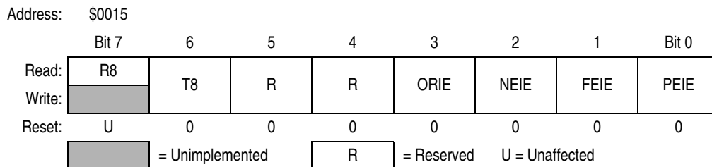
Figure 14-12. ESCI Control Register 3 (SCC3)
