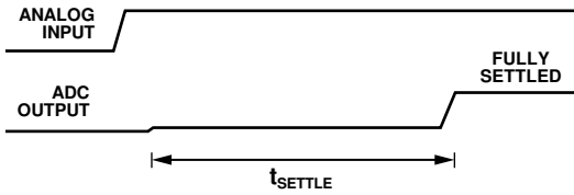
Figure 33. Step Input with Single Cycle Settling
