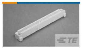
TE Part # CAT-313-PCB40 Free Height Plug Connector: Board-Board, Vertical, 40, 0.8mm TE Part # 5179029-1 0.8FH,P06H.5,040,08/Sn,TU
