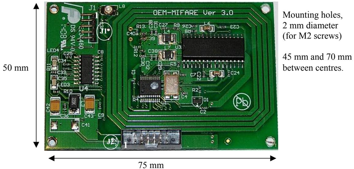
**OEM-MIFARE-ICODE-RS232 connectors** (note Pin 1 positions on diagram), note same J2 connector and pin out as USB version.
