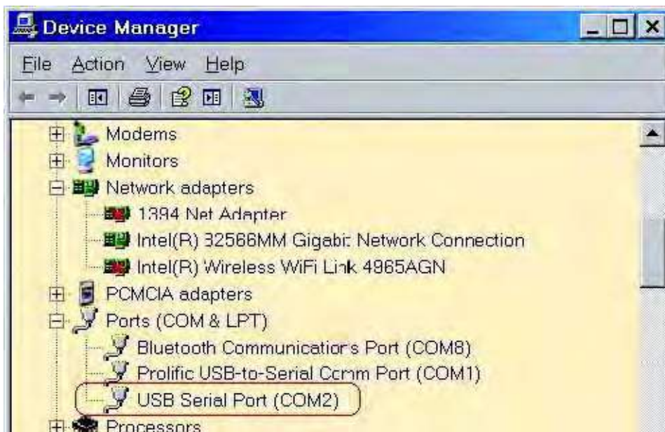
Figure 11. A Successful USB-to-UART Driver Installation
