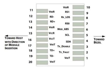
**Electrical Pin-out Details for SFP**
