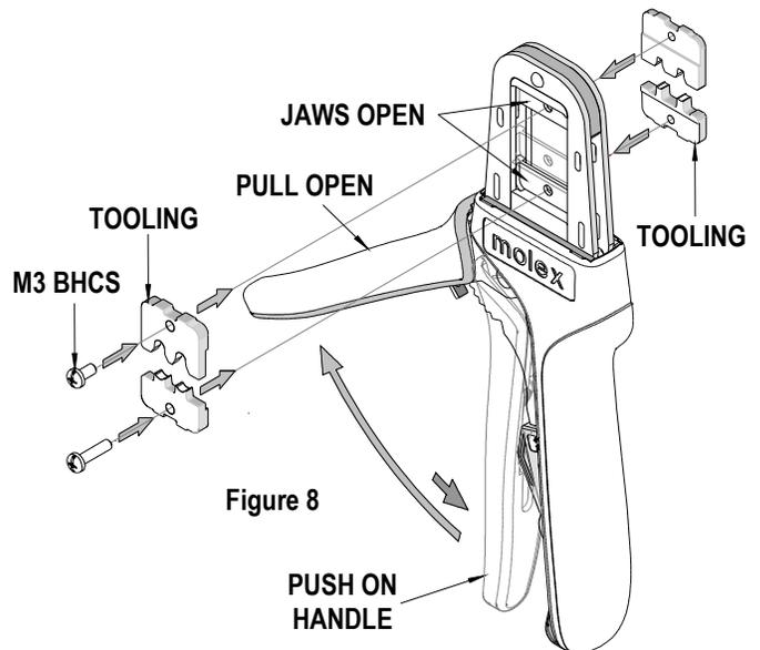
4. Do the same thing with the lower tooling and tighten the M3 screws. Be sure the small markings line up.
