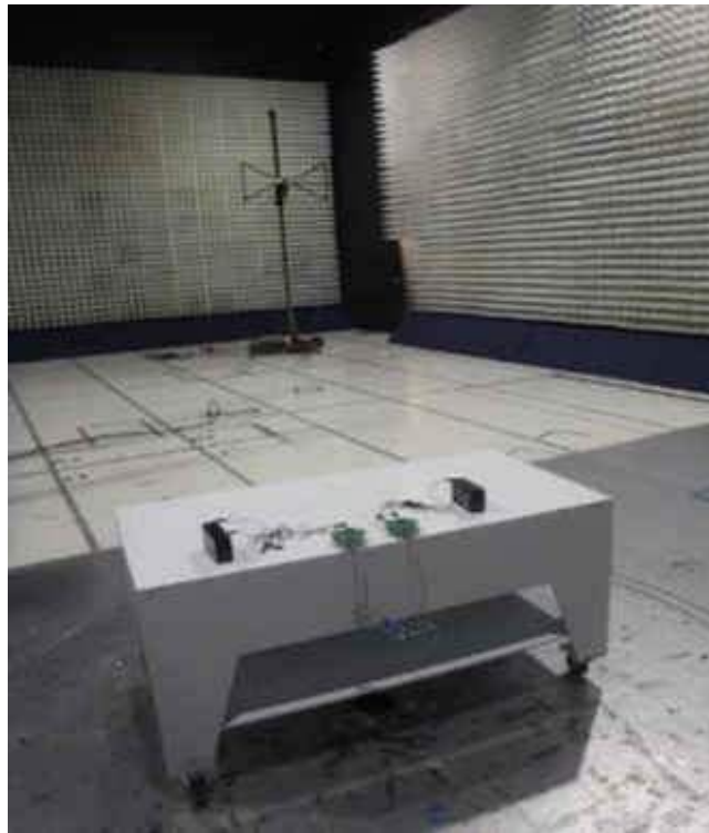
Figure 5-2. EMI Testing Setup in Chamber
