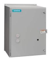
Mechanically held lighting contactor, Contactor amp rating 200Amp 0NC  $\_$  4NO poles, 110VAC 50HZ/120VAC 60HZ coil, Non-combination type, Encl NEMA type 4X 304 S-steel Water/dust tight noncorrosive
