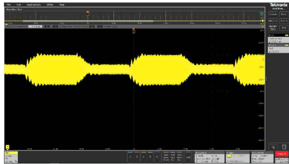
Figure 27. Transient Load on 15 V BUS
