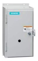
Non-reversing contactor, Size 2 1/2, Three phase full voltage, Contactor amp rating 60A, 3 wire (NO aux included), 240V 50Hz / 277V 60Hz coil, Non-combination type, Enclosure NEMA type 12, Dust/drip proof for indoors, Standard width enclosure
