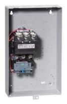
Non-reversing motor starter Size 3 1/2 Three phase full voltage Solid-state overload relay OLRelay amp range 50-200A 220-240/440-480VAC 60HZ coil Combination type Indoor general purpose use
