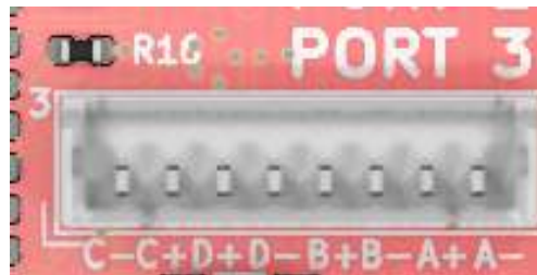
Figure 6: Ethernet port pinout
