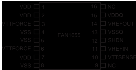
16-Lead Plastic eTSSOP-16 \theta_{JC} = 4^{\circ}\text{C/W}^*
