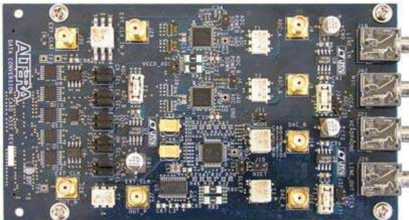
Figure 2. Cyclone III Data Conversion HSMC
