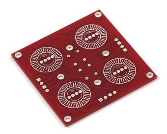
**Description:** This a simple breakout board for the button pads. Each LED and button is brought out to the side connectors. The connectors are soldered to the back side of the PCB. We recommend trimming the connector leads on the button side as short as possible to reduce the deflection of the pad.
