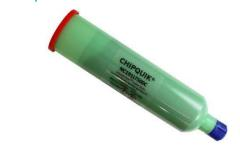
\*Shelf Life Notes: Chip Quik® solder paste is good past its quoted shelf life, regardless of refrigeration. Before use, visually inspect the solder paste to ensure it is not dried out or clumpy, or check stencil release. If stored in a jar, stir the product thoroughly for 2-3 minutes before inspection and use.
