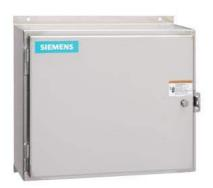
Mechanically held lighting contactor, Contactor amp rating 30Amp 0NC - 10NO poles, 208VAC 60HZ coil, Non-combination type, Enclosure NEMA type 12, Dust/drip proof for indoors
