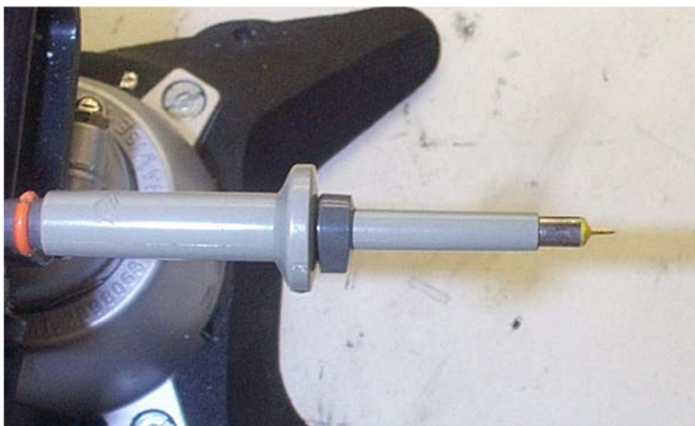
Figure 19 – Oscilloscope Probe Prepared for Ripple Measurement. (End Cap and Ground Lead Removed.)
