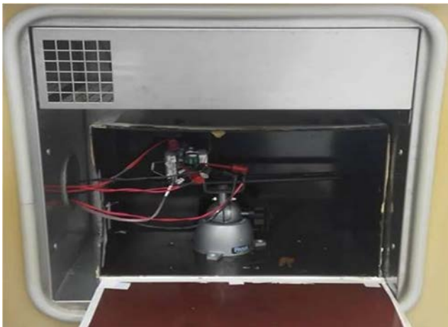
Figure 74 – Thermal Performance Set-up Using Thermal Chamber.
