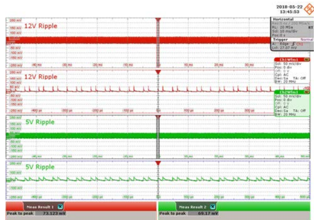
Figure 22 – 115 VAC Input. Vertical: 50 mV / div. Horizontal: 10 ms / div., 100 \mu s / div. 12 V Ripple: 73.123 mV PK-PK . 5 V Ripple: 69.17 mV PK-PK .
