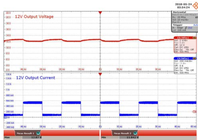
Figure 60 – 115 VAC Input. Upper: 12 V V_{OUT} , 2 V / div., 10 ms / div. Lower: 12 V I_{OUT} , 200 mA / div. V_{MAX} : 12.791 V. V_{MIN} : 11.921 V.
