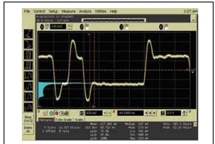
Output Waveform (400mV, 6dB pre-emphasis)
