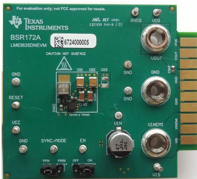
Figure 1-1. LM63635DNEVM Board Image
