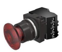
30mm BlackMax, Epoxy Coated Corrosion Resistant Complete Metal Unit Illuminated Twist-to-Release Full Voltage, 6V AC LED Lamp Mushroom Head Cap Small 1.79" (45 mm) Plastic Cap, Red 2 Position Maintained, Twist-to-Release with 1 N.O. - 1 N.C. Heavy Duty Contacts, A600/P600 UL Listed, CSA Certified NEMA 1,3,3R,4,4X,12,13 & Automotive Standards
