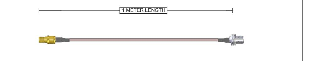
Connector A 132279 SMA Jack Straight Brass Gold + Heatshrink 50 Ohm RG-178 Continuity/Hi-Pot Connector B 172313 N-Type Jack Straight Bulkhead - Rear Mount Brass White Bronze + Heatshrink
