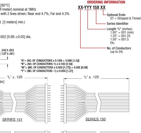
ALL DIMENSIONS: INCHES [MILLIMETERS] ALL TOLERANCES: ±0.005 [0.13] UNLESS OTHERWISE SPECIFIED CONSULT FACTORY FOR OTHER SIZES AND CONFIGURATIONS
