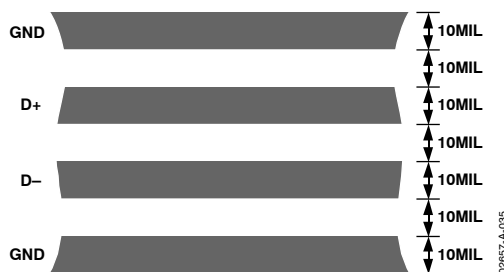
Figure 35. Arrangement of Signal Tracks
