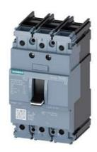
circuit breaker 3VA5 UL frame 125 breaking capacity class S 25kA @ 480 V 3-pole, line protection TM210, FTFM, In=50A overload protection Ir=50A fixed short-circuit protection Ii=10 x In UL489 SB (naval), 50 deg. cel. cable connection on both sides
