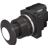
30mm BlackMax, Epoxy Coated Corrosion Resistant Complete Metal Unit Illuminated Push-Pull Operator Transformer type, 480V AC Incandescent Lamp Mushroom Head Cap Small 1 3/4" (44.5 mm) Metal, Black with White Lens 2 Position Maintained, Pull-to-Release UL Listed, CSA Certified NEMA 1,3,3R,4,4X,12,13 & Automotive Standards
