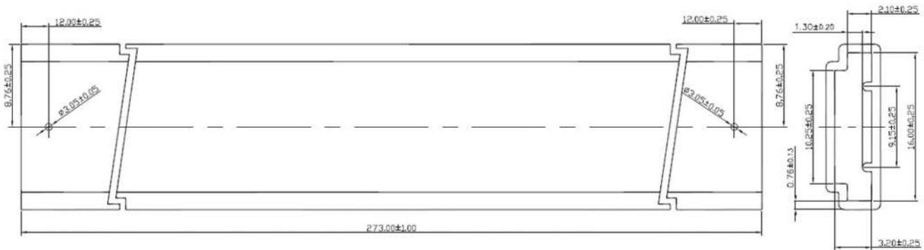
Figure 9. Tube dimensions for LUXEON CoB Compact Range (Gen 2).
