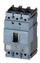
circuit breaker 3VA5 UL frame 125 3-pole, starter protection TM120M, AM, In=1A without overload protection short-circuit protection Ii=5...12 x In cable connection on both sides
