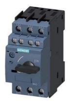
Circuit breaker size S0 for motor protection, CLASS 10 A-release 1.4...2 A N-release 26 A screw terminal Standard switching capacity with transverse auxiliary switches 1 NO+1 NC  $\,$
