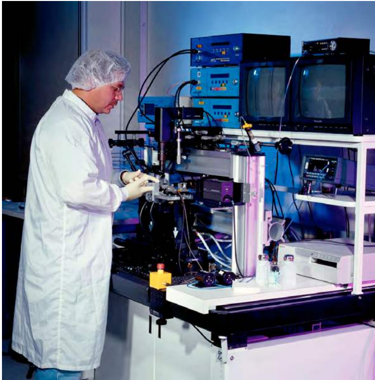
Photo 3. A technician prepares to align and position a single-mode optical fiber with a laser. The very small dimensions of single-mode optical fiber require very precise positioning equipment.
