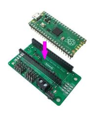
Power is provided via a terminal block connector, the supply is then controlled by an on/off power switch to the board. There is a green power LED to indicate when the board is turned on. The power connections are reverse polarity protected.
