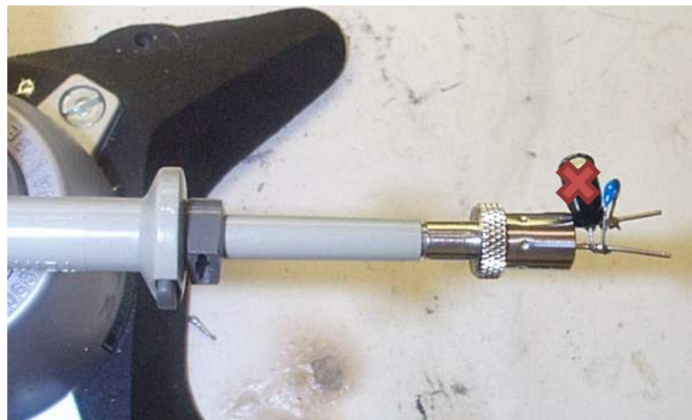
Figure 43 – Oscilloscope Probe with Probe Master ( www.probemaster.com ) 4987A BNC Adapter. (Modified with wires for ripple measurement, and one parallel decoupling capacitor added)
