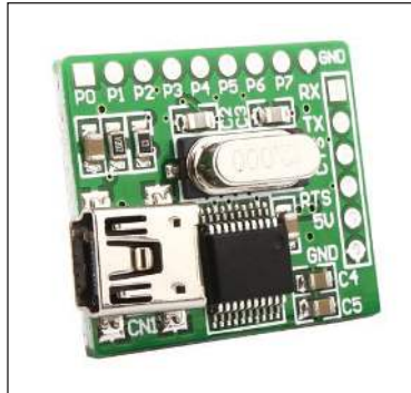
Figure 1: USB UART 2 additional board
