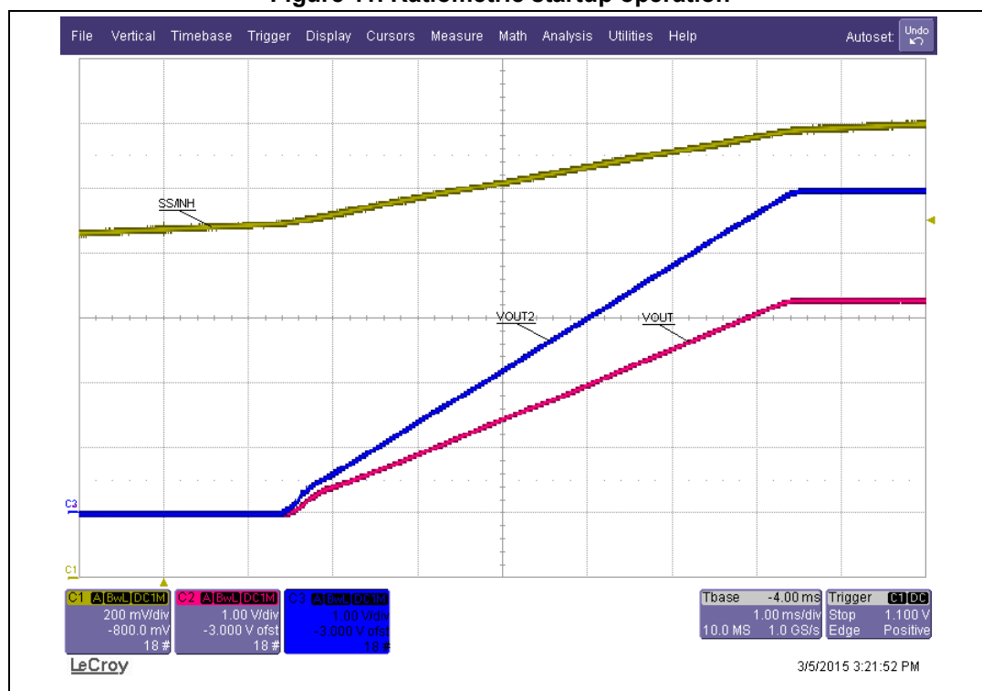
Figure 11. Ratiometric startup operation
