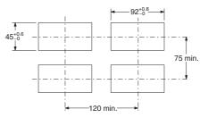
Note: The values above are recommended values. Do not group-mount the meters at intervals less than the recommended ones.
