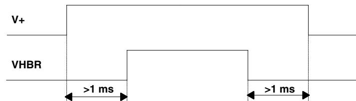
Figure 3–1. Recommended Power-Up and Power-Down Sequence
