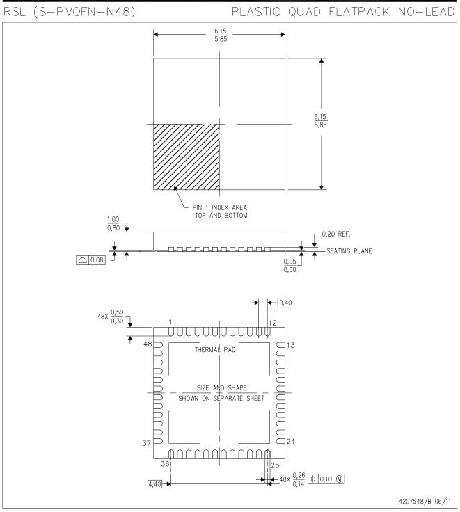
NOTES: A. All linear dimensions are in millimeters. Dimensioning and tolerancing per ASME Y14.5M-1994.
