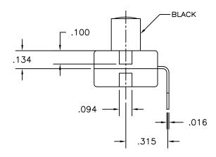
JUDCO INVENTORY NO. 50-0101-00 SWITCH TYPE: PUSH BUTTON, SPST, ON-OFF ELECTRICAL RATING: 12VDC, 500mA
