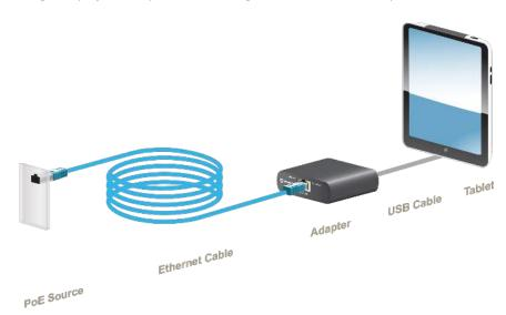
Microchip PoE to USB-C adapter connects USB-C devices to the PoE network and converts both power and data into a single USB-C connector.
