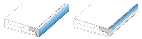
The front optical surface is not allowed to be blocked by the host system. In x direction the entire surface is used by the sensors optics.
