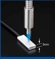
The UV intensity can be relative measured\* at the actual position by using the slim UV sensor. It can also automatically adjust the UV intensity to the preset level. Since the sensor only has 5 mm (0.2 in) thickness, which is similar to the workpiece, the intensity measurement is possible without removing the system from the production line, facilitating
