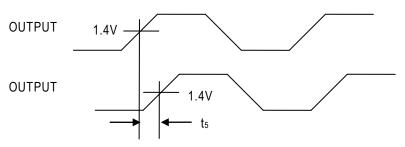
**Input-Output Propagation Delay**
