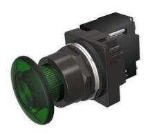
30mm BlackMax, Epoxy Coated Corrosion Resistant Complete Metal Unit Illuminated Push-Pull Operator Transformer type, 600V AC Incandescent Lamp Mushroom Head Cap Small 1 3/4" (44.5 mm) Plastic, Green 3 Position Momentary UL Listed, CSA Certified NEMA 1,3,3R,4,4X,12,13 & Automotive Standards
