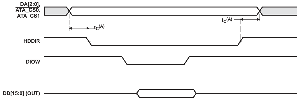
Figure 6-38. ATA/CF HDDIR Taskfile Write/Single PIO Write Timing
