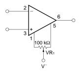
★ Remark The OFFSET NULL pins should be left open or connected to V<sup>-</sup> via a resistor as shown in the left figure. Don't connect to any lines other than V<sup>-</sup>, otherwise mulfunction, degradation, or failure may occur.
