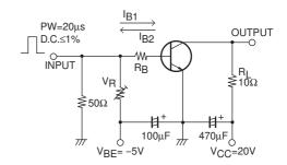
$20I_{B1} = -20I_{B2} = I_C = 2A$ For PNP, the polarity is reversed.
