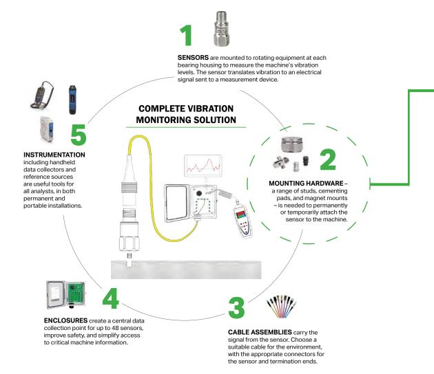
Wilcoxon offers complete vibration monitoring solutions for permanent sensor installations or walkaround monitoring. Permanent sensors offer consistency and simplified access to data, while temporary installations allow greater flexibility, usually at a lower cost.
