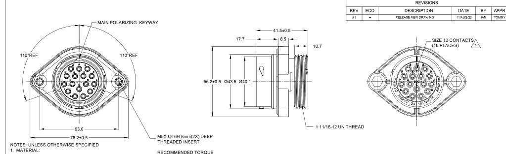
2. MODIFICATIONS: WIDE THREAD ADAPTOR (WTA); STANDARD DIA. WIRE SEAL SEALED PANEL MOUNT
